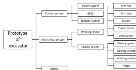
Figure 3. Composition of prototype
