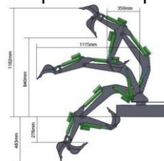
Figure 5. Working space of prototype
