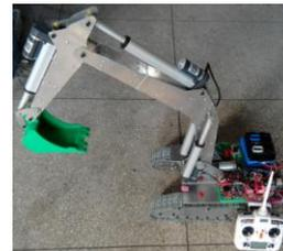
Figure 10. Prototype of excavator
