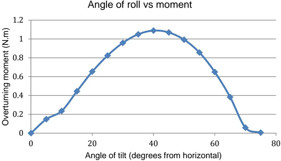
Figure 7: Graph of overturning moment vs angle of tilt as measured by a student group of their vessel.
