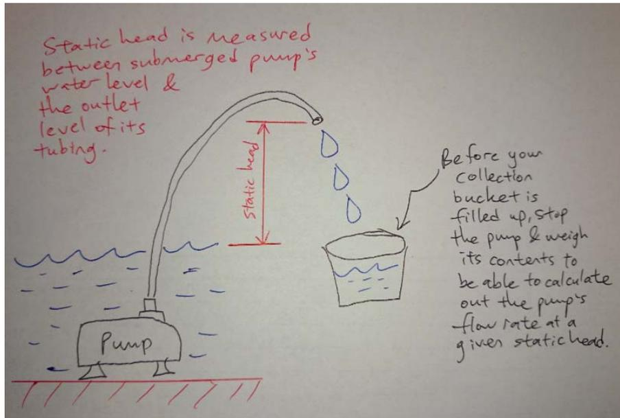
Figure 4. Pump characterization experiment setup diagram as written down for students.
