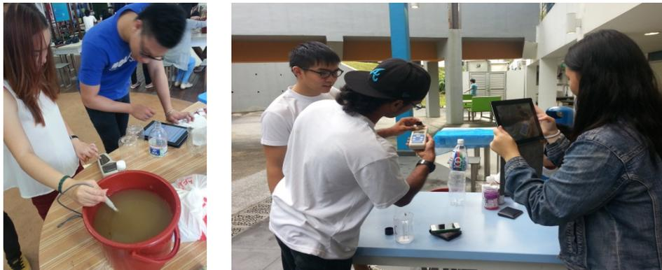
Figure 8. (left) Measuring the pH and turbidity of dirty water, (right) measuring the pH and turbidity of filtered water
