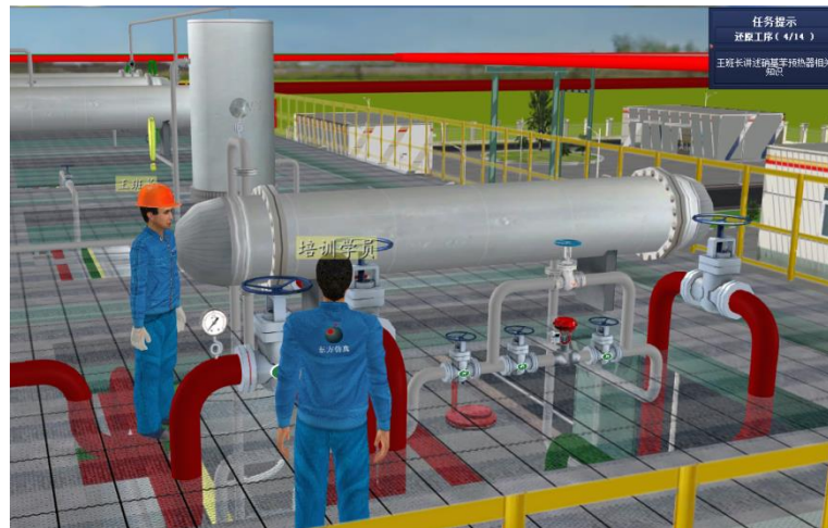
Figure 2. The interface of 3D virtual simulation for phenyl amine fluidized bed device
